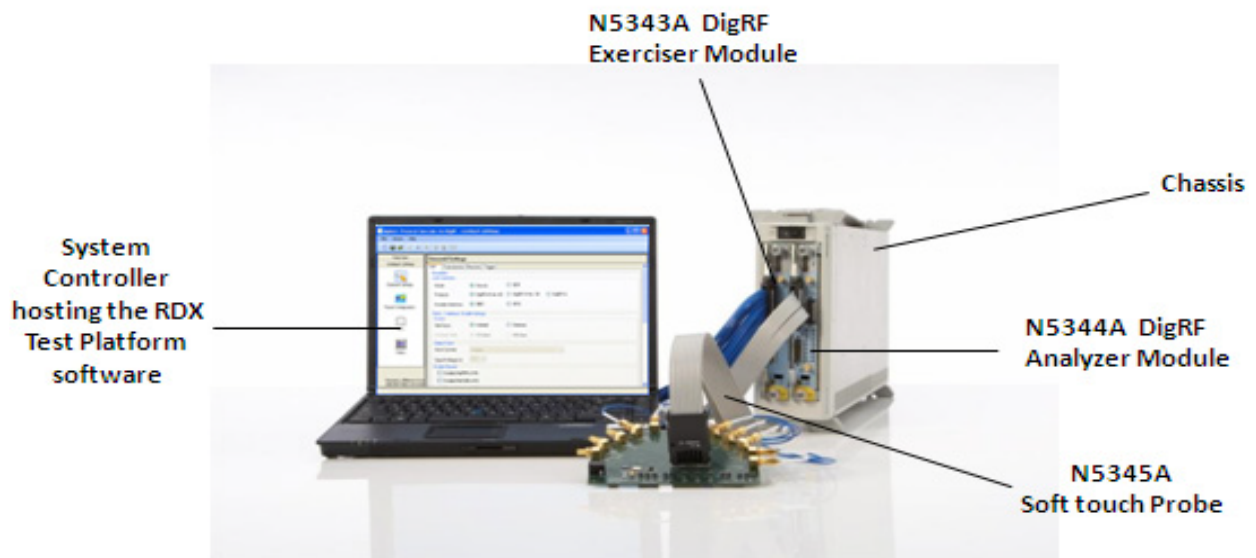
Figure 1 RDX Test Platform Components
